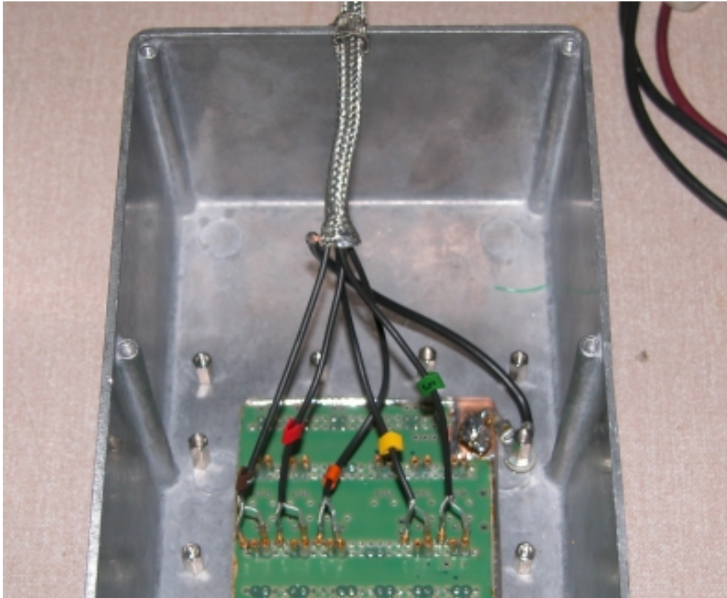
Figure 3. Close-up of coaxial umbilical connection to motherboard
