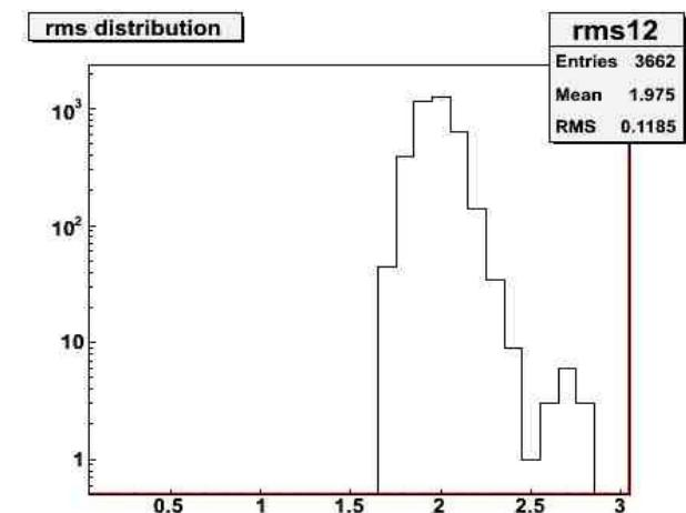
Comment: All channel are electronically operational. The tail of the RMS distribution for G12 is due to channels with long connecting cable from the VPT to the mother board.
