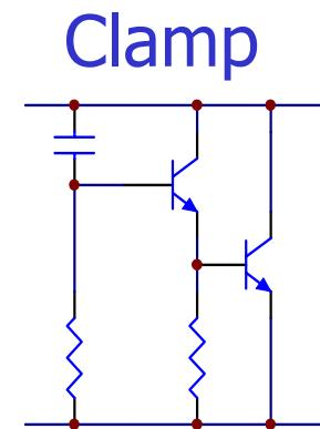
Transient clamps from  $V_{CC}$  to  $V_{EE}$  (analog and digital)
