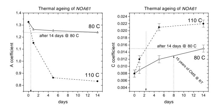
Assuming the Arrhenius low, from A: 14days @  $80C \equiv 0.5day$  @ 110 C C: 14days @  $80C \equiv 2.3days$  @ 110 C  $\Rightarrow E_a(A)/k = 15000 \text{ K} E_a(C)/k = 8140 \text{ K}$ A: 15 years @ RT = 0.9 day @ 80 C  $\Rightarrow A = 1.269$ C: 15 @ years @ RT = 8 days @ 80 C  $\Rightarrow C = 0.013$
