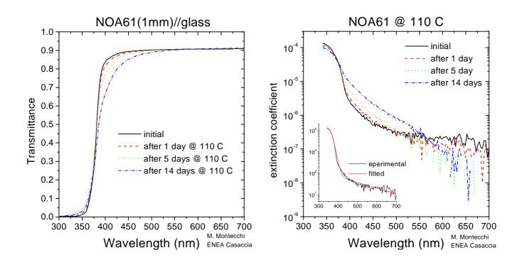
Two different ageing processes modify the transmittance spectrum: the first acts on the slope (+), the second on the knee (-); they are well described, respectively, by A and C coefficients of
