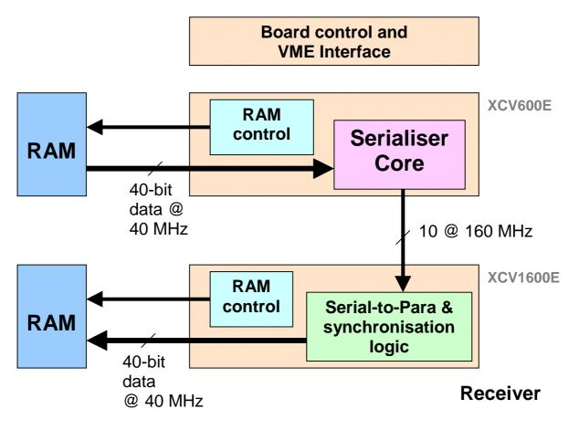
Test Real-time data path; serial-to-parallel conversion @ 160 MHz, Xilinx DLLs.
