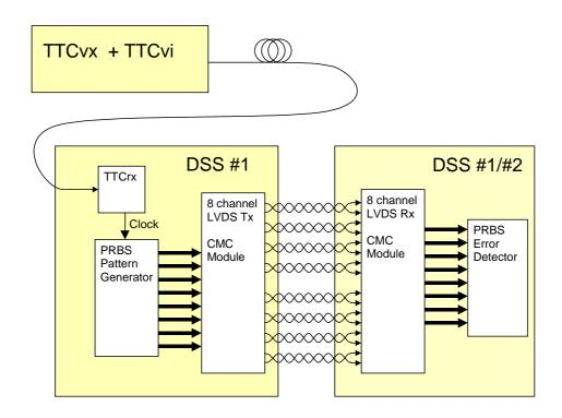
Results using the original LVDS deserialiser DS92LV1210 operating at 40MHz (maximum frequency) showed a low tolerance to power supply noise and clock jitter. (March 2000)  $\rightarrow$
