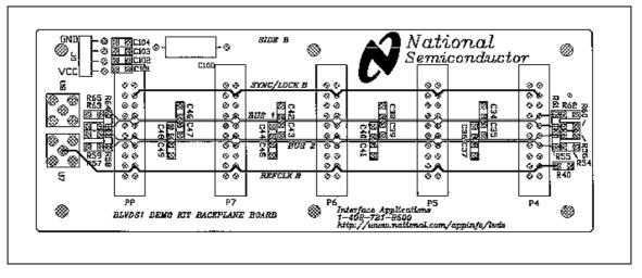
Each side of the backplane card has 2 differential busses, a REFCLK bus to distribute the REFCLK signal to deserializer cards, and a SYNC/LOCK bus that connects the LOCK\* output from deserializers to the SYNC1 input of the serializer.
