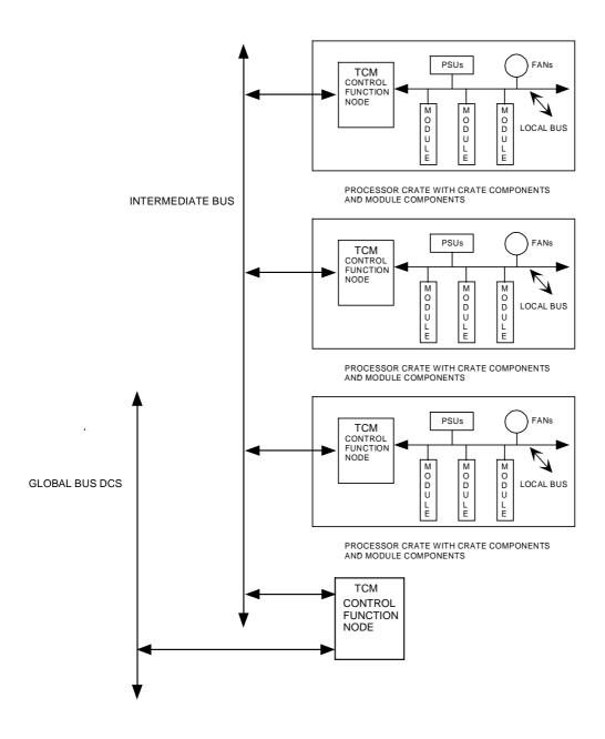
LEVEL 1 TRIGGER CRATES PLUS THE 'LOCAL', 'INTERMEDIATE' AND 'GLOBAL' BUSES
