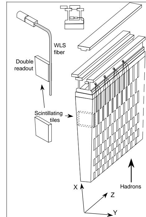
Figure 1: Conceptual design of a Tile calorimeter module.
