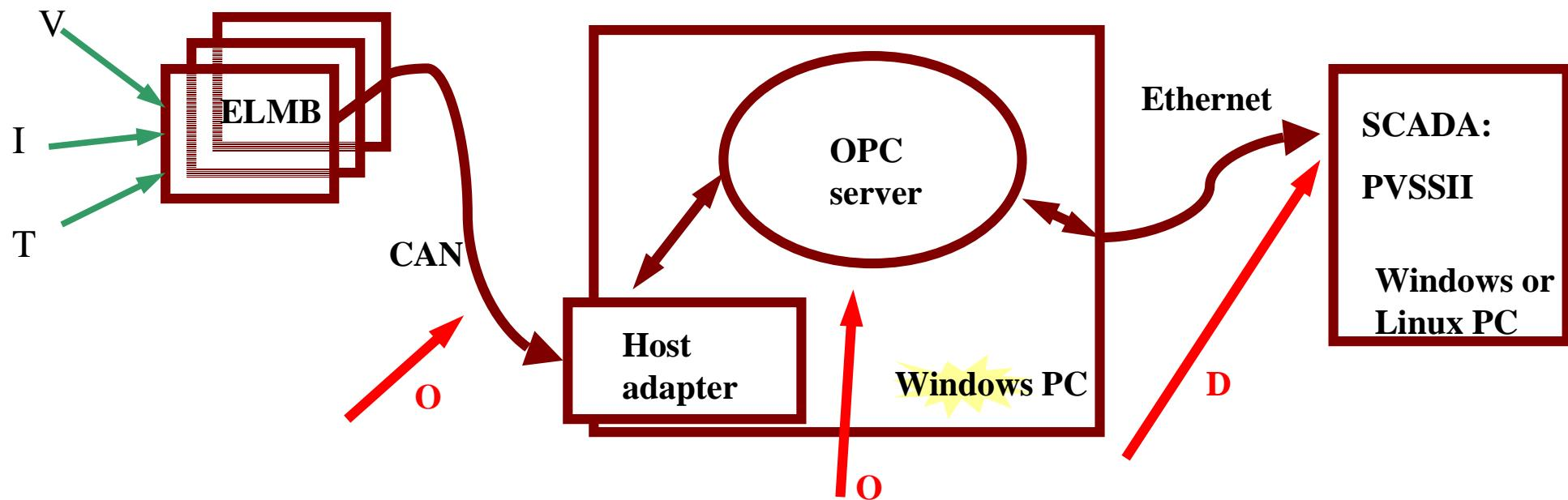
Software and firmware for standard components available from ATLAS DCS group. To feed non-standard user data into the chain we need our own OPC server (O) or PVSS drivers (D)
