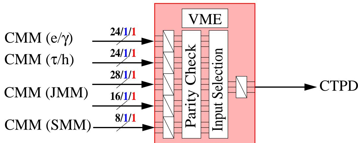
⇒ total input signals: **108 trigger inputs + 5 clock + 5 parity**
