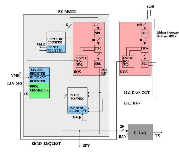
• RoC controls and reads out local RoS which located in the processor FPGAs
