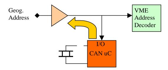
More robust design ... add resistors in series with CAN uC 'inputs'.
