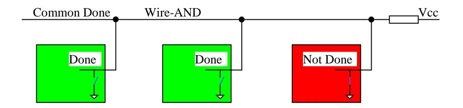
However, XILINX FPGAs signal 'configuration completion' by releasing the DONE pin ... and then wait for this pin to be released externally! Not very good for fault tolerance, development work ...
