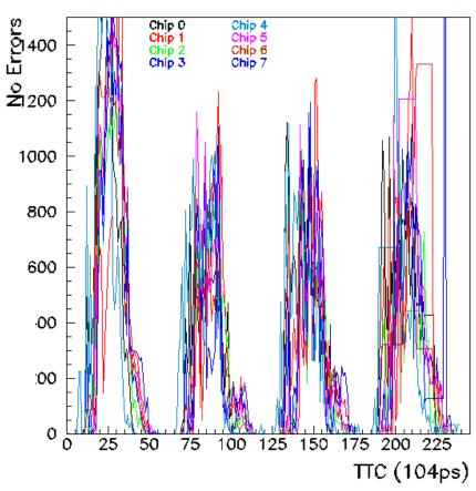
Total error, with BP, as a function of CP chip clock.
