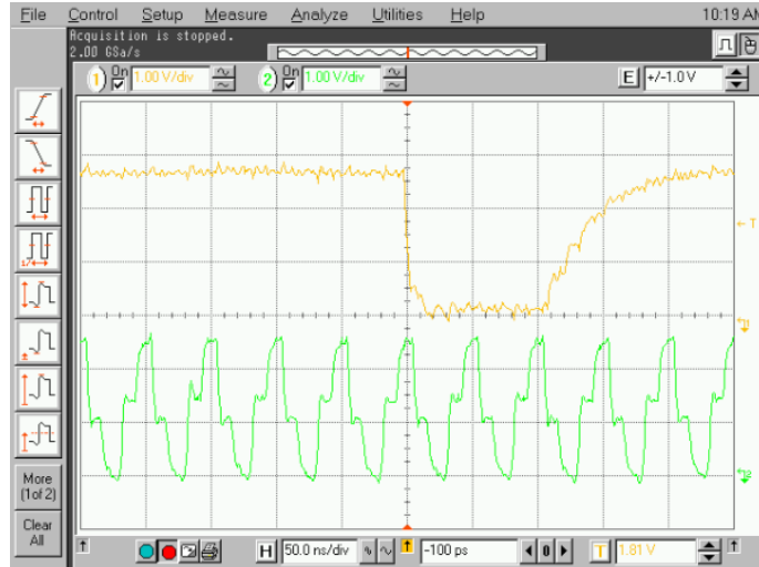
Figure 7: Measured cross talk between the VME bus and merger lines. The DTACK signal (yellow) is asserted at the end of a VME cycle. A repeating signal on one of the longest data merger lines (green) is unaffected by the VME activity. The time scale is 50 ns/div, and the vertical scale is 1.0 V/div for both traces.
