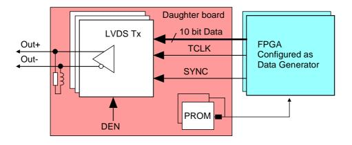
The installed pre-compensation will be for 15m - 20m of cable of type similar to AMP part# 1370754-1. The pre-compensation R & L are easily changed to accommodate different cable lengths and types.
