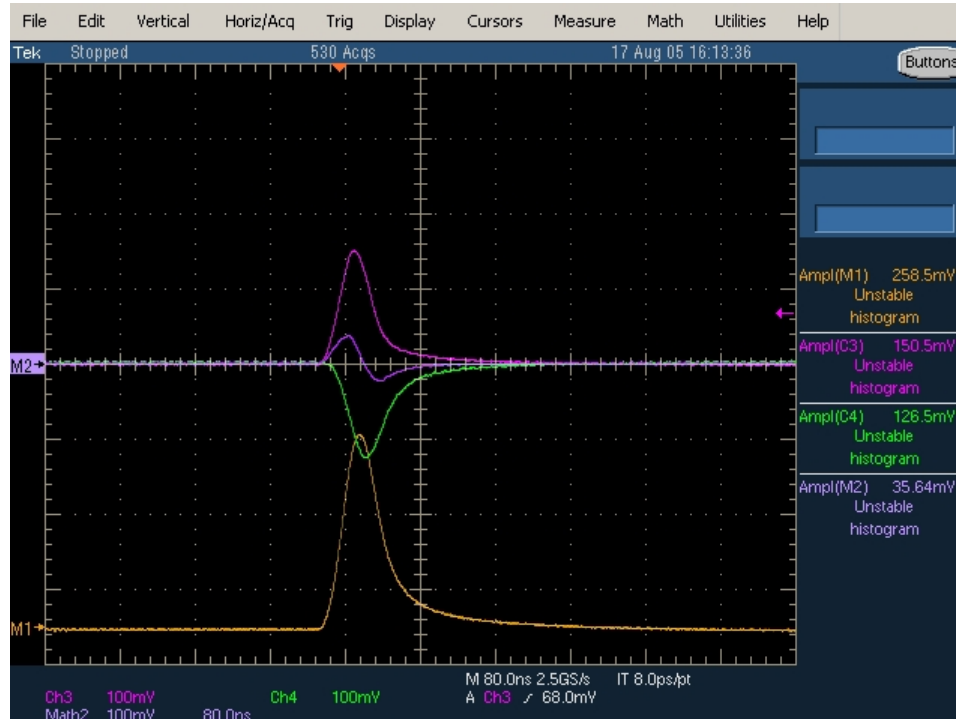
Figure 16: Response of Turquoise/Brown + White pair to triangular pulse input
