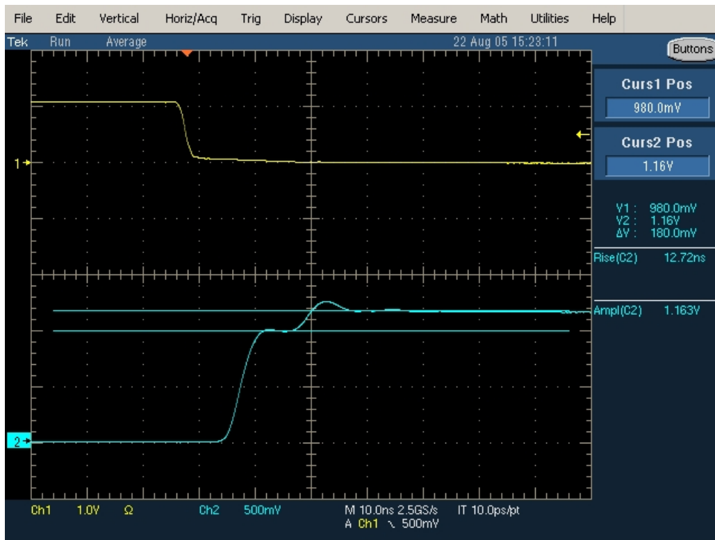
Figure 17: TDR waveform for differential impedance measurement of LAr analogue cable
