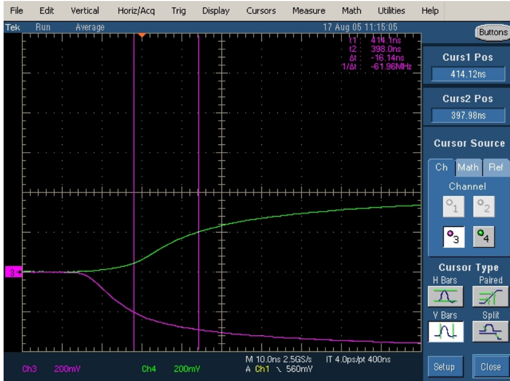
Figure 13: Differential mode skew for Turquoise/Brown + White pair
