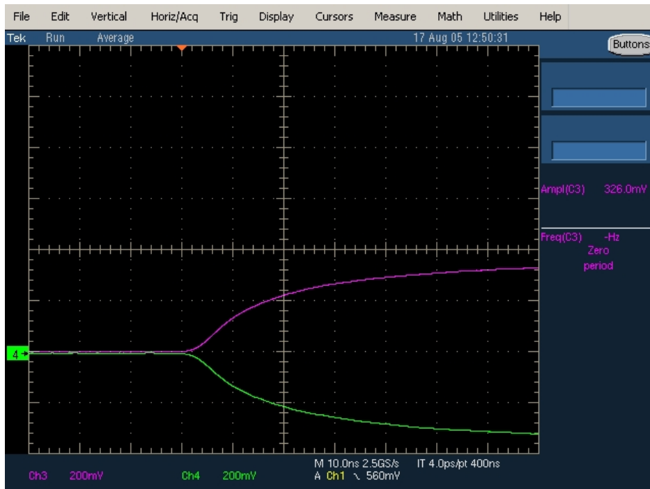
Figure 11: Differential mode intra-pair skew for Purple + White Pair
