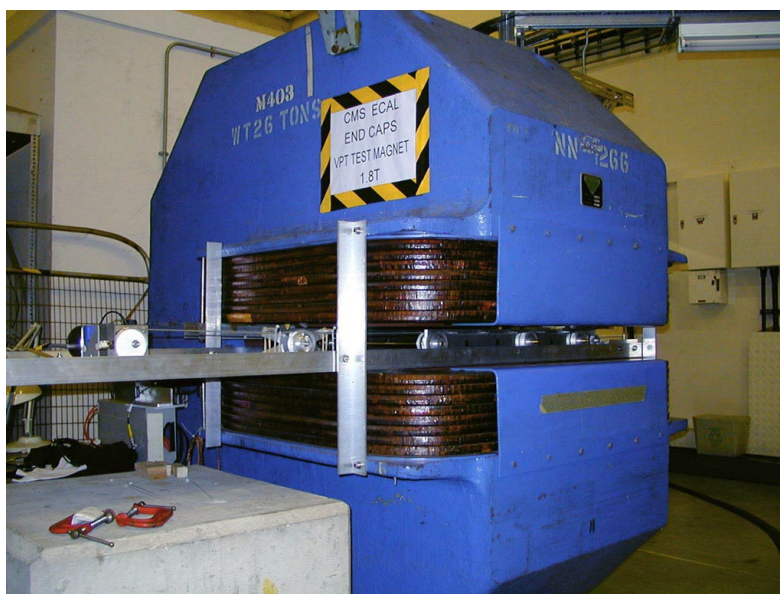
Figure 11. The 1.8T test rig at RAL.
