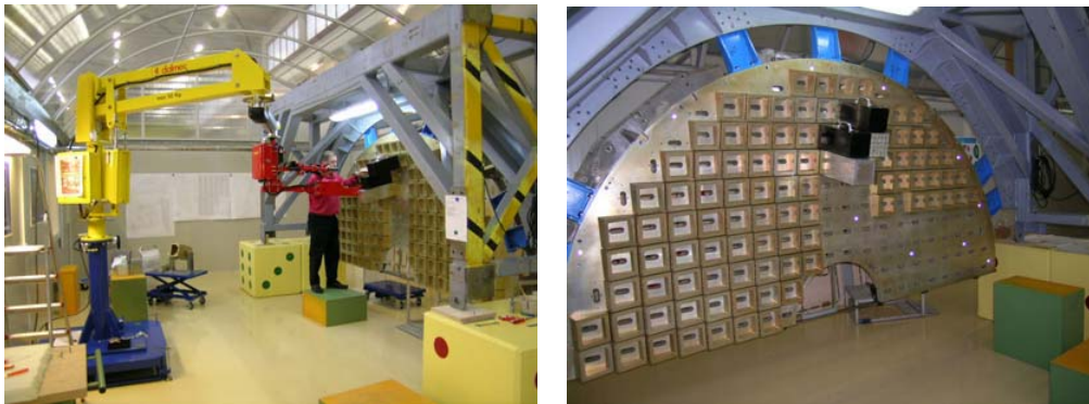
Figure 5. A Dee under preparation in the Crystal Palace at CERN, and, right, a Dee with its set of positional spacers with 4 SCs under trial mounting.
