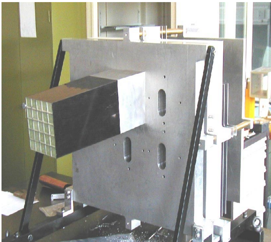
Figure 20. The prototype section of a Dee, E0', with a capacity for 4 Supercrystals
