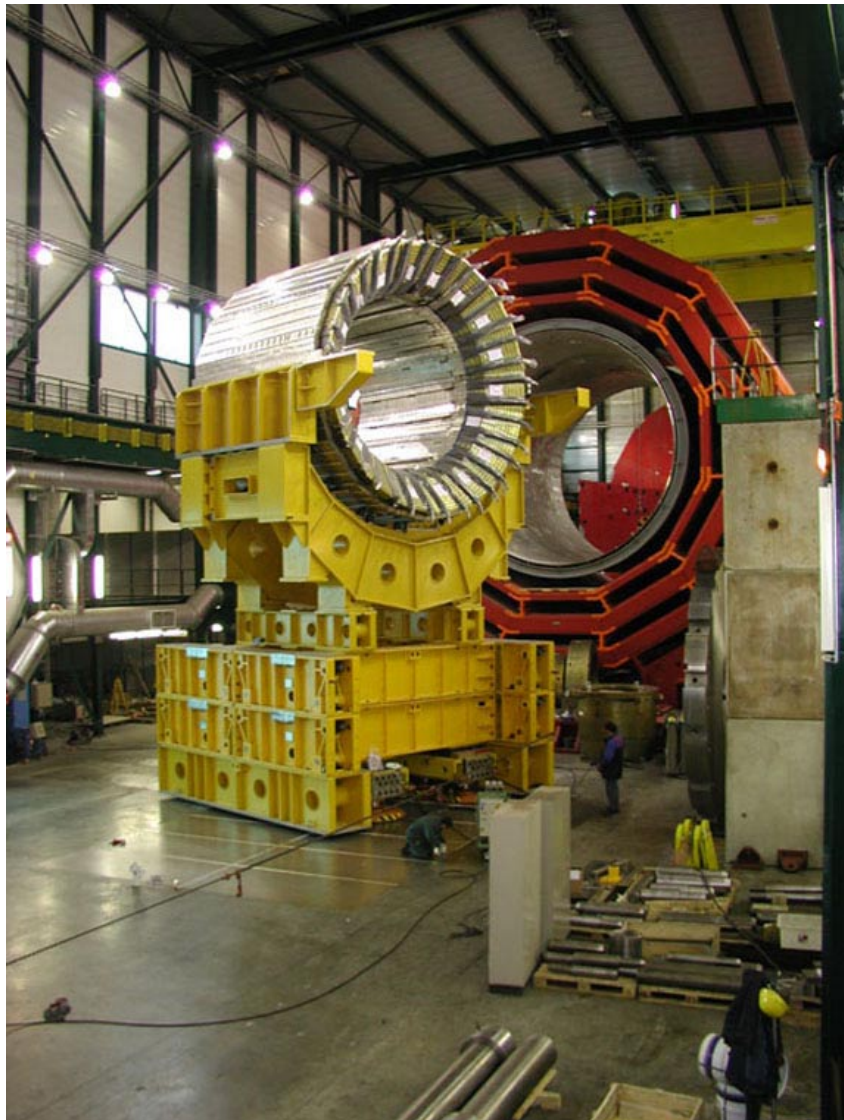
Figure 1. The first half-barrel of the CMS HCAL, assembled at Point 5. The assembled Barrel section of the magnet yoke can be seen in the background
