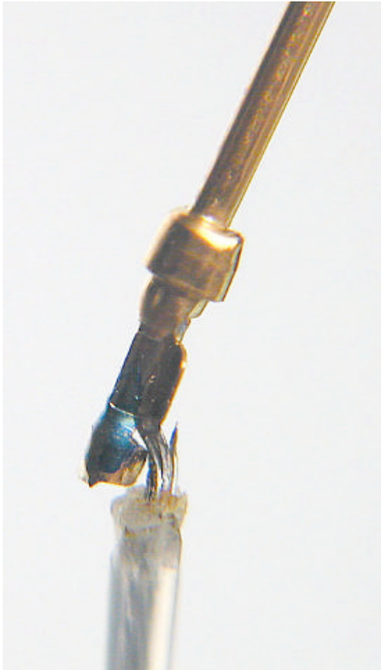
Figure 1. VPT 539 - poor crimping of pin to flying lead
