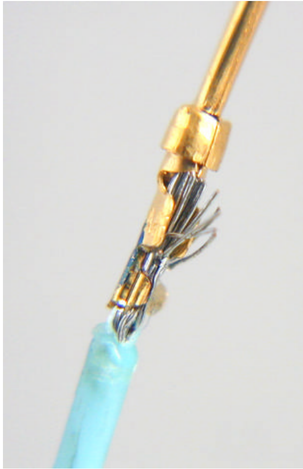
Figure 2. VPT 560 - poor crimping of pin to flying lead
