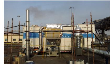
Electron beam tests at a power station in Poland. (Right) accelerator; (above) beam delivery.
