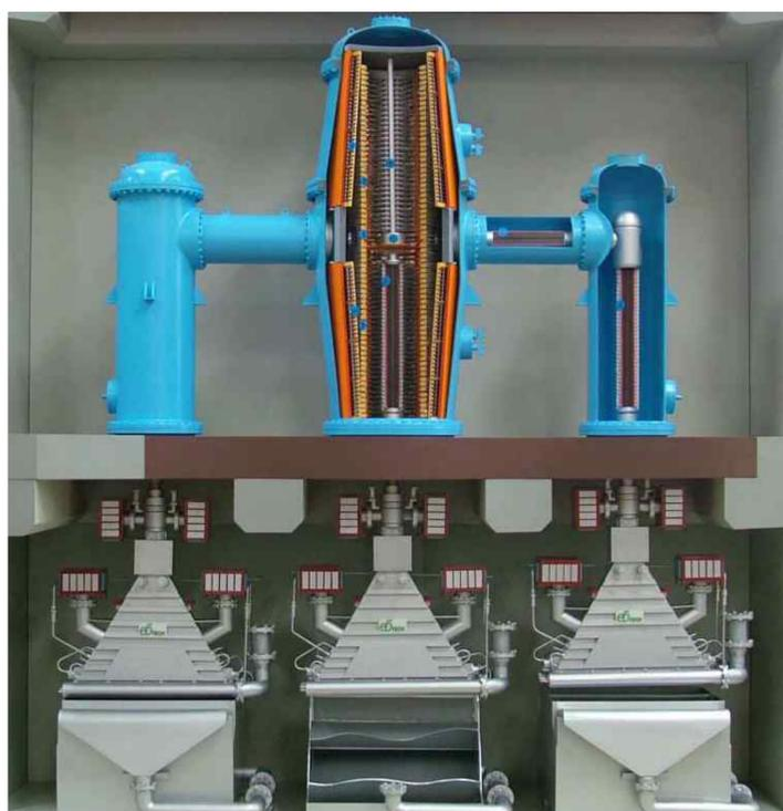
A facility in Korea used for removing dye from waste water
