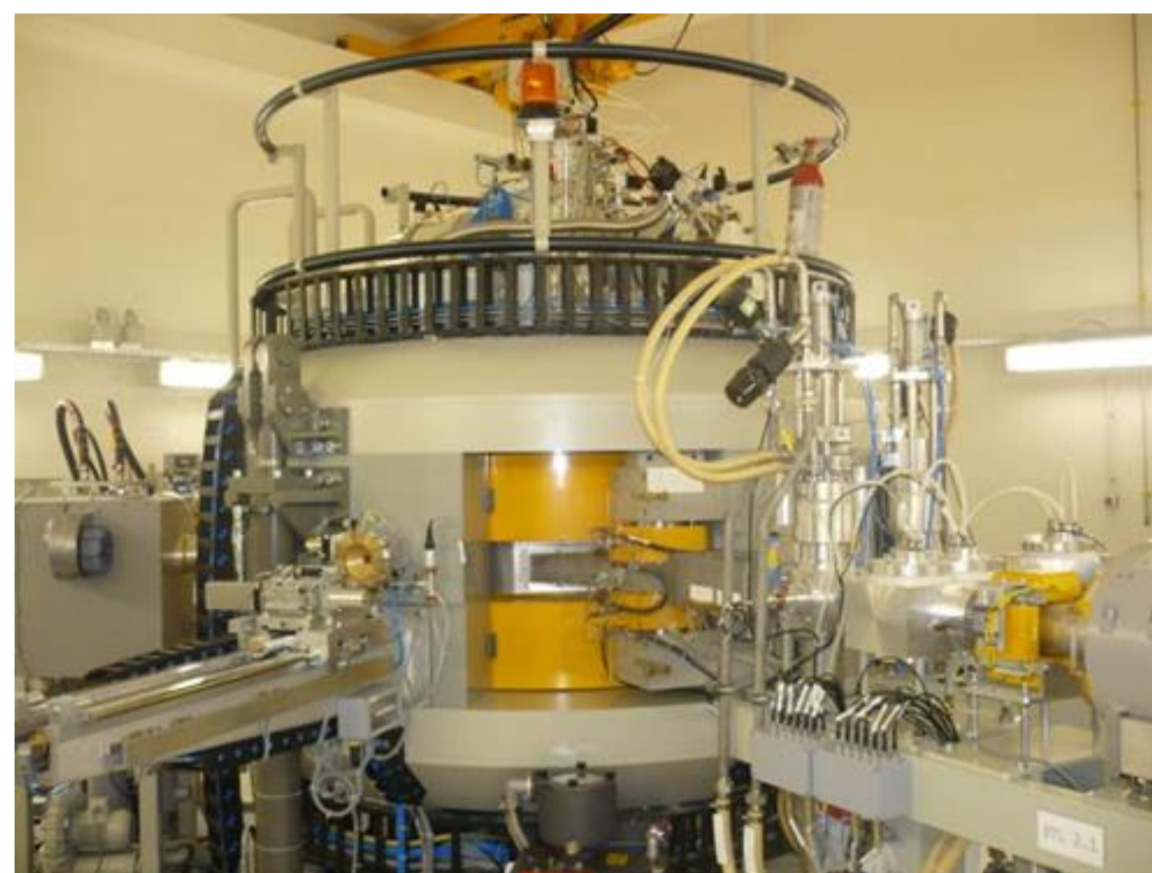
A 30 MeV radioisotope production cyclotron manufactured by IBA of Belgium
