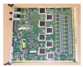
Figure 3: Example of a CPM processor module
