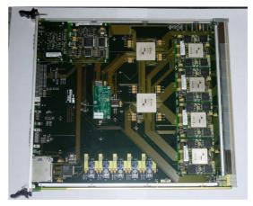
Figure 4: Example of a JEM processor module
