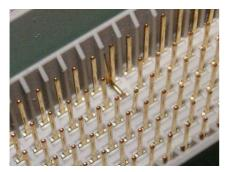
Figure 7: Photograph of damaged connector
