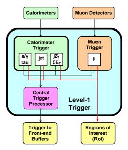
Figure 1: ATLAS Level-1 Trigger
