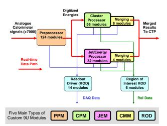
Figure 2: Level-1 Calorimeter Trigger
