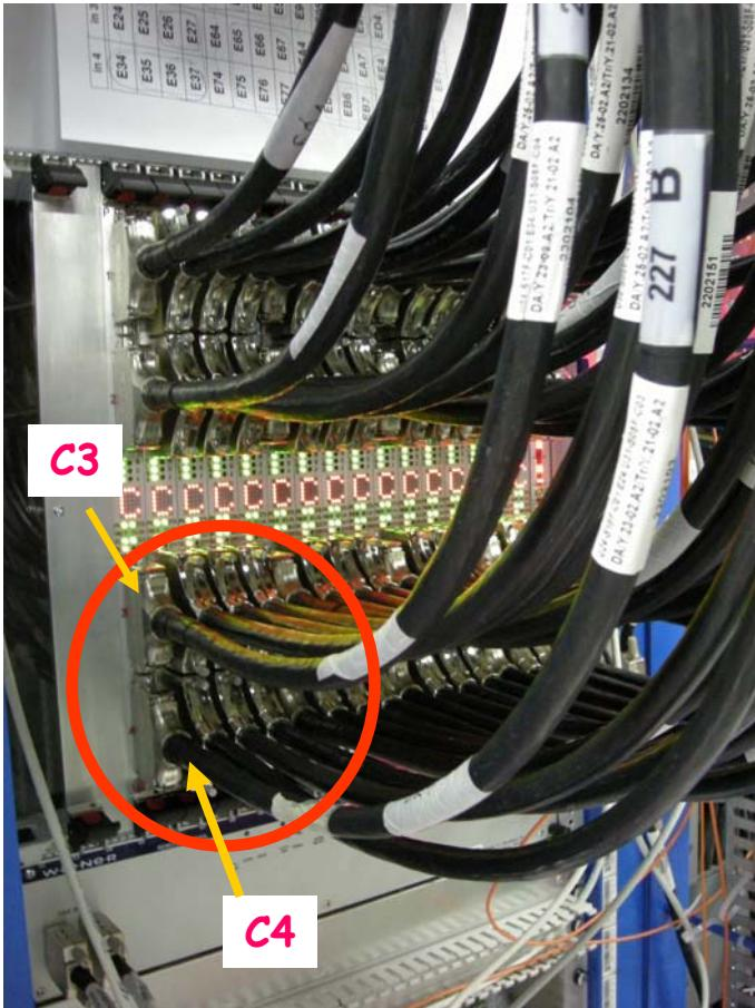
Mistake was corrected by swapping the cables at PPM input
