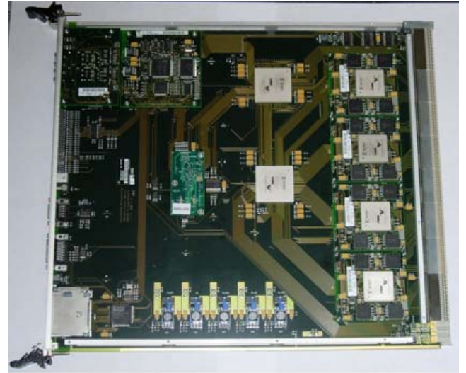
Fig. 5 Photograph of a production Jet/Energy Module (JEM)
