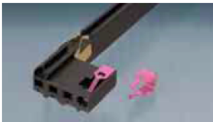
Figure 1: Bottom “foot” of the crate guide rail. The three square holes are used for module keying.
