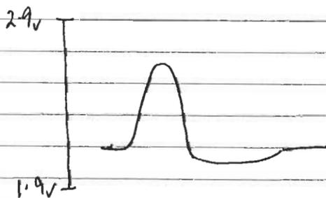
DAC: 1.7 to 2.15 V ( $\sim$  500 mV range) 8 bits, 2 mV/count.
