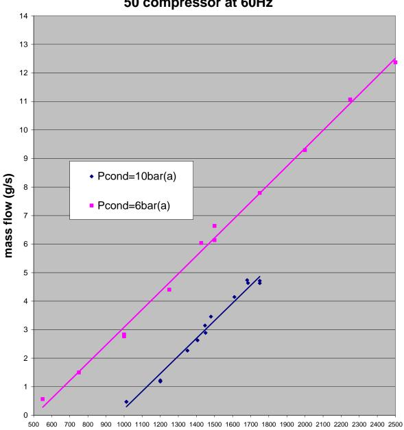
C3F8 mass flow vs Inlet pressure for Haug SOGX 50 compressor at 60Hz
