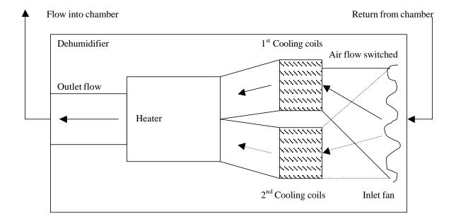
Basically the air is drawn in on the right hand side, through a filter. It is then directed through *one* of the sets of cooling coils. These run in tandem with the hot vapour return from the set in use being passed through the stand-by set. This hot vapour de-frosts the unused set and prepares it for its next stint. It is this process that floods the floor if you don't have a bucket to hand!
