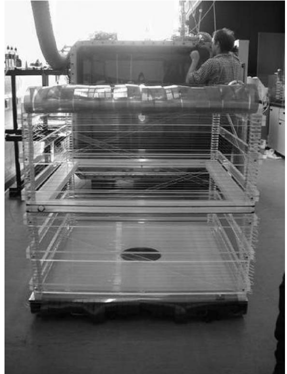
Fig. 2. Picture of the DRIFT-I detector, showing the main detector outside and in front of the vacuum vessel.
