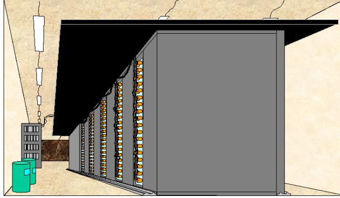
Figure 8. Schematic drawing of a half kton LS module in the WIPP. The lead doors enclosing the ends are not shown so that the location of the PMTs may be seen. The muon veto detectors are seen at the top.
