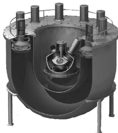
Fig. 3. Cut-away illustration of the single phase ZEPLIN I liquid xenon detector showing target arrangement within the liquid scintillator Compton veto. Not shown is the lead gamma shielding.
