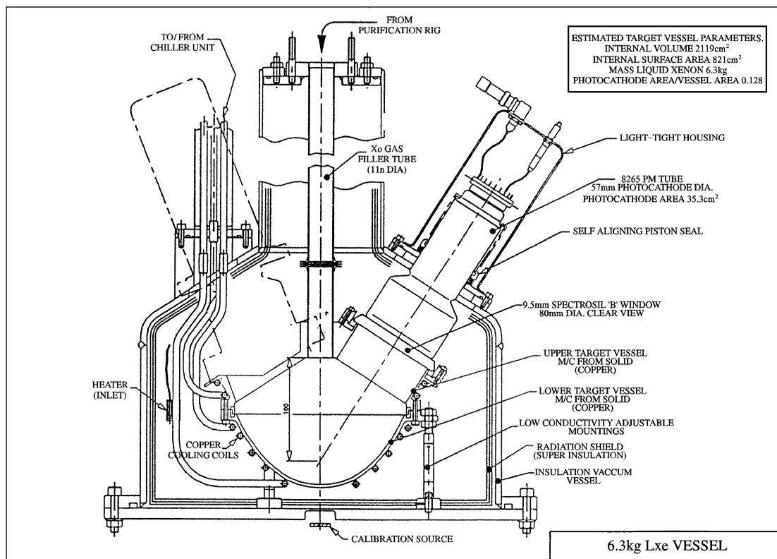
Fig. 4. Single-phase liquid Xe detector.
