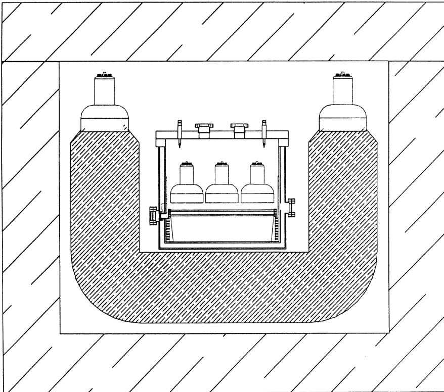
Fig. 5. Two-phase ZEPLIN detector in scintillator veto.
