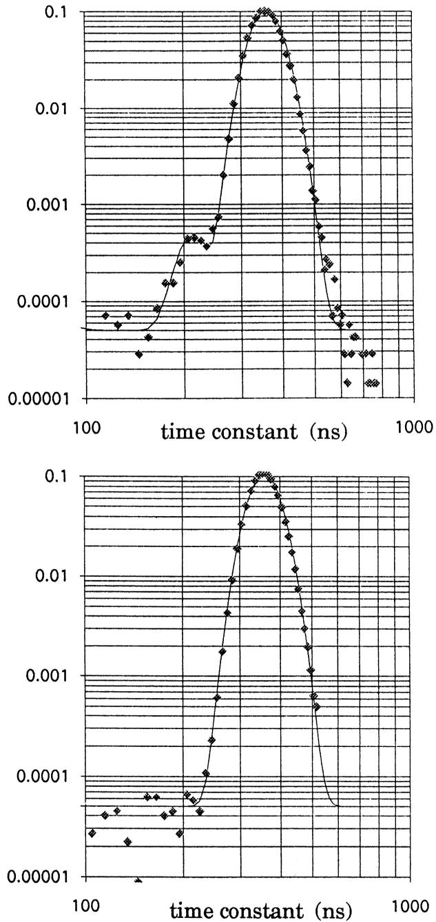
Fig. 1. Time constant distributions (normalised to unity) for 5 kg NaI crystal: (*upper graph*) Background distribution showing additional population of shorter pulses; (*lower graph*) Compton calibration with  $^{60}\text{Co}$  source (5 h each day).
