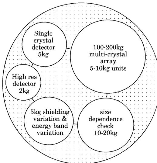
Fig. 3. Array of NaI detectors for diagnostic studies of signal-like events.
