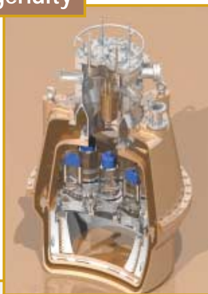
A cut-away drawing of the new ZEPLIN II detector currently being constructed
