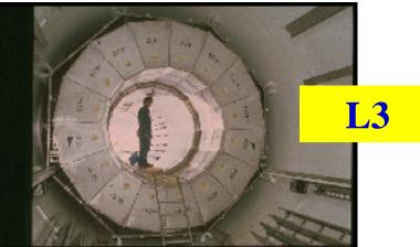
Alternating layers of steel and streamer chambers
